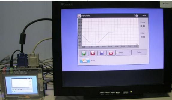
Figure 27 : Data Logger - Graph Display
