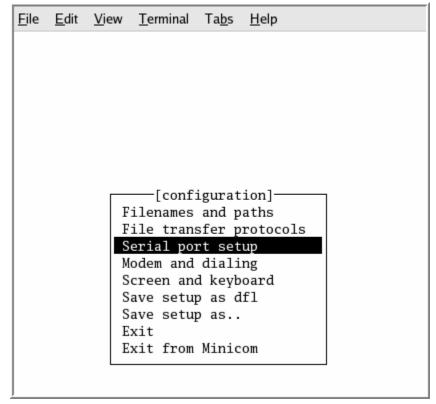
2. Select the Serial Device, baud rate and other parameters as shown in Figure 16. Here, we have selected Serial device as /dev/ttyS0 but it may differ as per your development machine.
