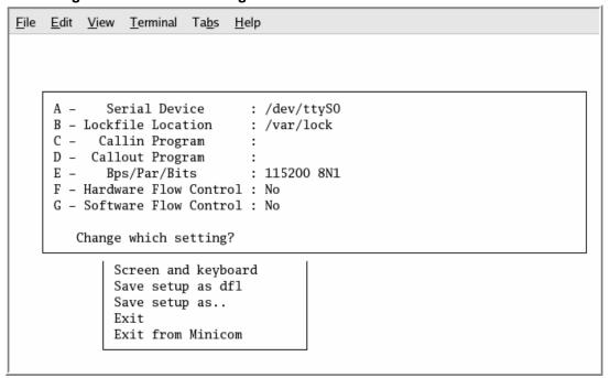
3. Set the baud rate 115200, 8 bit, no parity and one stop bit. See the Figure 17
