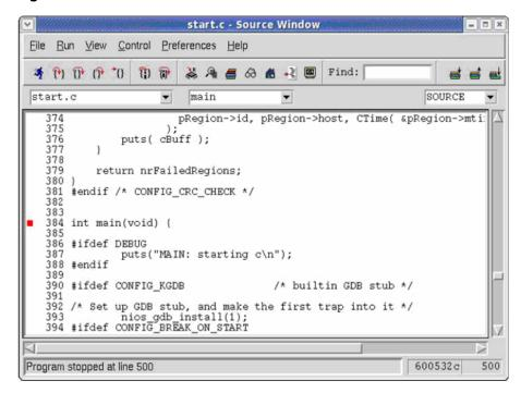
Now you can debug easily with aid of GUI. You can set the break point, check the content of registers and see the assembly code also.
