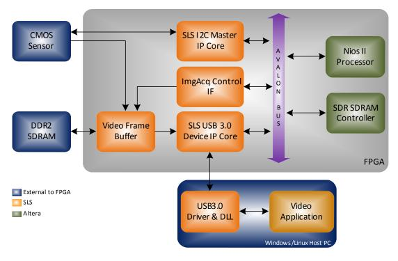
As shown in the block diagram, a CMOS camera sensor data is being transferred over USB 3.0 interface using SLS USB 3.0 Device. The Nios II processor is used to control peripherals such as memory controller, I2C master and enumeration of the USB 3.0 Device on Host PC running with Windows or Linux Operating System (OS).
