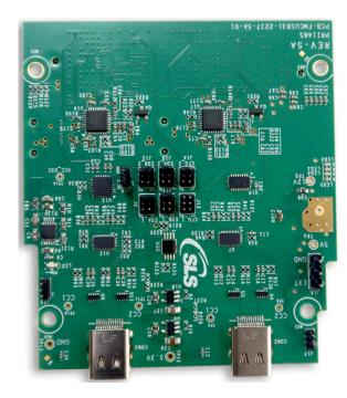
The following example shows the USB 3.2 FMC connection with FPGA Development Kit.
