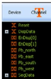
4. We need to capture at least 100 or 90 seconds of data (80 seconds for one timer cycle and other 20 or 10 seconds for viewing the next cycle beginning). If we set the sampling rate as **100 MHz** (default), then our memory **128Kbits** will get filled up in **0.128** seconds only. Therefore,
